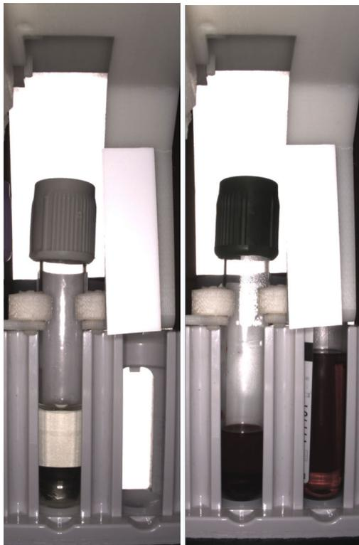
As part of the process design, JADAK provided the customer with a recommendation on the container background. The material and position of the container, as well as illumination, can have a significant impact on the reliability of results. JADAK recommended a plate behind the spinner on the backside to provide the background needed for optimal image capture.
