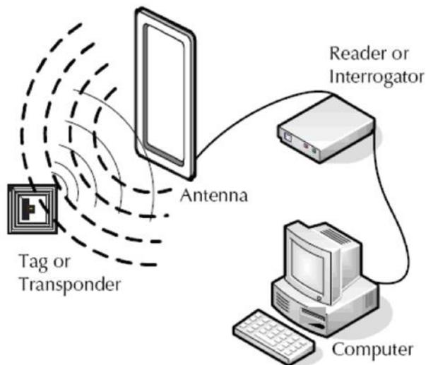
**RFID Tag** -- RFID tags or labels are embedded with a transmitter and a receiver. The RFID component on the tags have two parts: a microchip that stores and processes information, and an antenna to receive and transmit a signal. The tag contains the specific serial number for one specific object.
