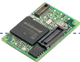
Decoding Board (DB-206) is miniature decoder board that can be used with JE-233V.
